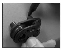
C. Then, insert a single well-nut into each mounting hole. Insert the small end first so that the rim of the "top hat" on the other end prevents the well-nut from going all the way through.
