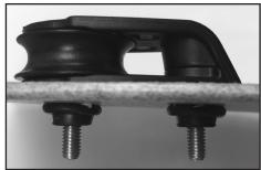
**DO NOT** apply any form of silicone caulk to the well-nuts during this process. The well nuts are designed to mushroom out as they compress to create a water-tight seal. The use of sealants is not necissary and could actually prevent the well-nuts from sealing properly in which case leaking could occure.
