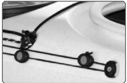
Take the loose piece of shock cord and tie a knot in one end. Thread the shock cord through one of the toggles, through and round the front deck fitting and back to the other toggle. Tie the shock cord off to the second toggle leaving the line under tension.
