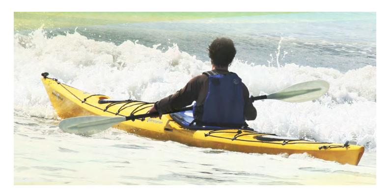
Length: 353 cm / 11'7" Width: 65 cm / 25.75" Boat Weight: 20 kg / 44 lbs Max Capacity: 114 kg / 250 lbs Deck Height: 36 cm / 14" Cockpit Length: 90 cm / 35.5" Cockpit Width: 50 cm / 19.75"
